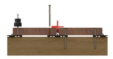
entilation pads can be used to prevent water and moisture from trapping between the prisms and terrace boards and the associated potential risk of rot.
